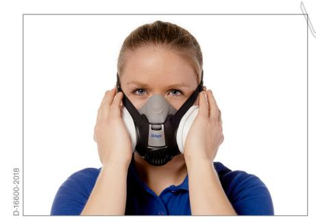
Negative pressure test: Seal both respiratory filters with your hand and breathe in until a negative pressure is created. Hold your breath for a moment. The negative pressure should be maintained. If not, adjust the harness.
