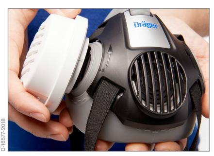
Ensure that the line markings on filters and mask line up. Insert the filters in the direction of the arrow until they lock into place.
