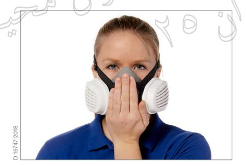
Positive pressure test: Seal the exhalation valve of the half mask and breathe out forcefully. The half mask must not lift off your face. If the exhaled air dissipates between face and mask body, adjust the harness.
